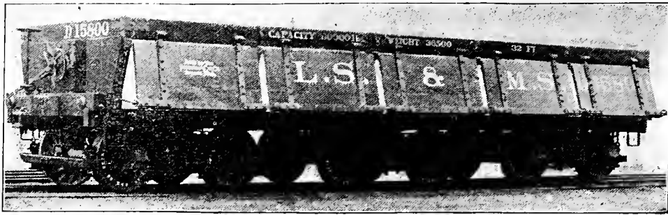
Fig. 27. SIDE-DUMP ORE CAR. LAKE SHORE & MICHIGAN SOUTHERN RAILWAY. Length, 32 ft. Capacity, 80,000 lbs. Weight, 36,500 lbs. (Details are shown in Figs. 332-335.)
